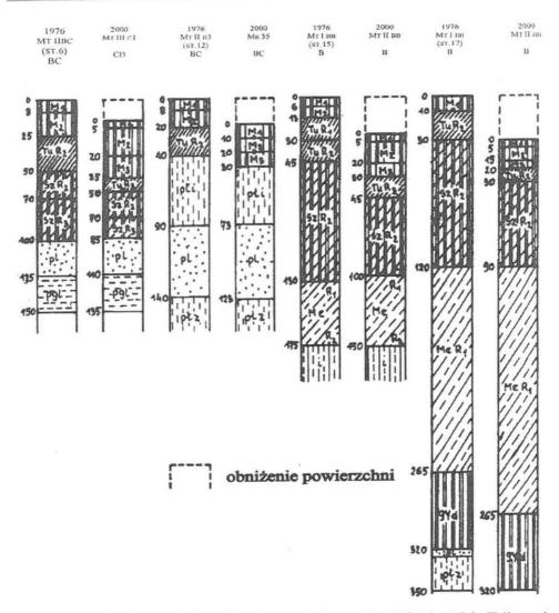
Fig. 1. Morphological characteristics of intensively dehydrated soils MtIIbc (loc.16) in Zbójno and MtIIb3 (loc.12), MtIbb (loc.15), MtIbb (loc.17) in Zienki in the period 1976-2000
